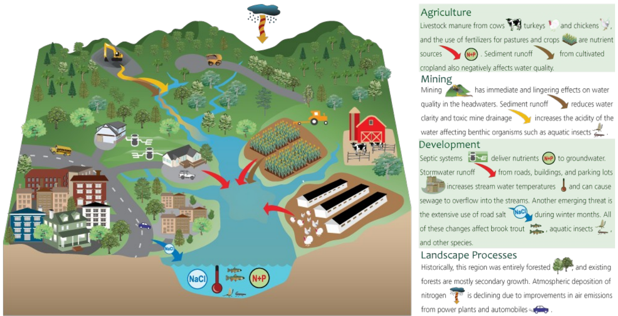
Figure 3: Conceptual diagram of a watershed.
